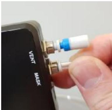
*Inserting pressure tube*
