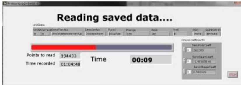
Downloading may take up to 5 minutes, depending on the amount of data. When downloading is complete the SE-RDA unit will switch itself OFF automatically. The data is now loaded in the SE-RDA software and appears in the main window, but it is *not yet saved to disk*.
